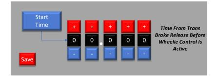
Note: To use the Profiler Wheelie Control, you must set Profiler Channel-1 to Parameter 4 (Pitch) to activate. See Profiler Channels in the next section for details. When the VPS is connected to a Profiler (not PFEFI), you can also record any 2 channels on the Profiler and view them in the software. This is extremely useful for evaluating the acceleration performance of the car during the run. Determining when Longitudinal G is rising or falling is key to tuning the Profile to the proper levels.
