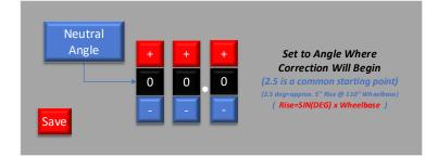
VEHICLE POSITION SENSOR WWW.MORETRACTION.COM The angle at which the VPS will begin to send a signal to start dropping cylinders (SmartDrop) is also adjustable as well as the maximum level of SmartDrop, if any.
