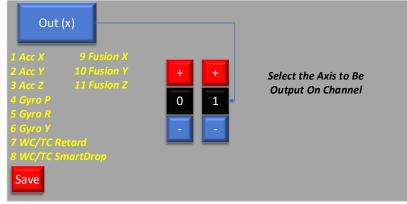
Acc X = Longitudinal Accel Acc Y = Lateral Accel Acc Z = Vertical Accel Gyro P = Pitch Gyro R = Roll Gyro Y = Yaw WC/TC Retard = Wheelie/TC Retard WC/TC SmartDrop = Wheelie/TC SmartDrop Fusion X = Fusion Pitch Fusion Y = Fusion Roll Fusion Z = Fusion Yaw Fusion is only to be used when vehicle not running
