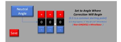
VEHICLE POSITION SENSOR WWW.MORETRACTION.COM <u>Output Limit</u> is the maximum amount of timing that can be retarded and is also adjustable. This setting is useful to limit the total retard that the Wheelie Control can retard on different systems. For example, a 100% Retard correction on FuelTech is 35 deg of ignition retard, if you never want to retard more than 15 deg., then you would set the limit to 42%.
